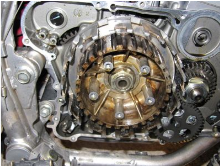
Burned out KLR clutch caused by the heavy mud.
